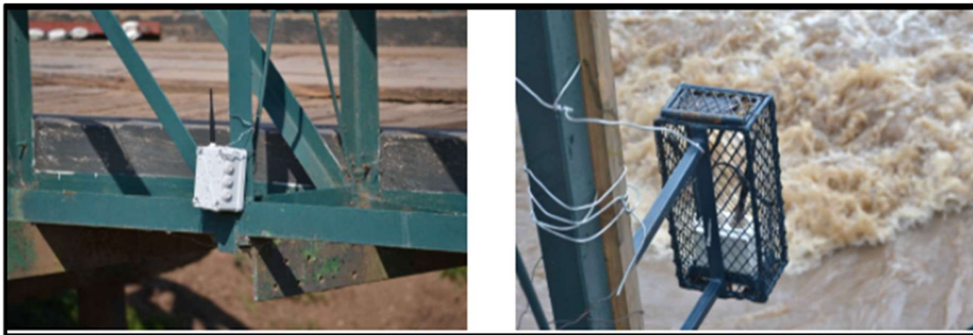
Figure 4: Deployment (Prototype on the Left was destroyed by Baboons and the One on the Right has a primate proof cage)
