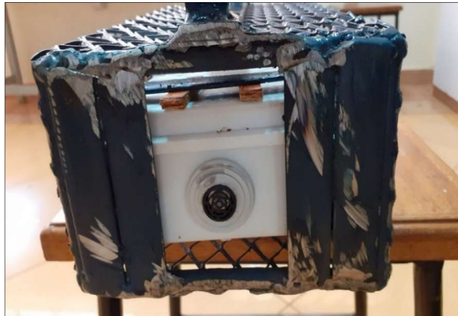
Figure 7: MB1010 Ultrasonic sensor location
